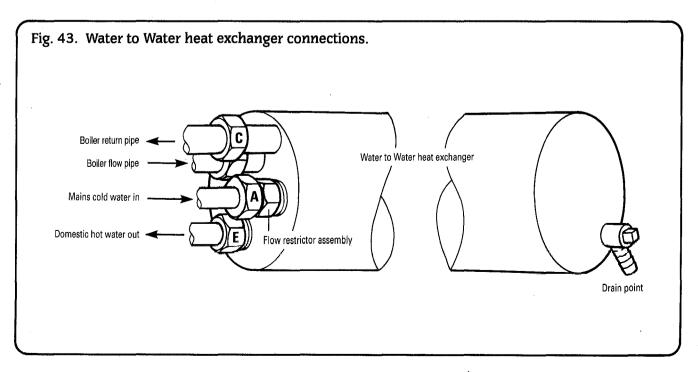
Note. The direction of flow should be downwards. The speed should always be set to maximum.
