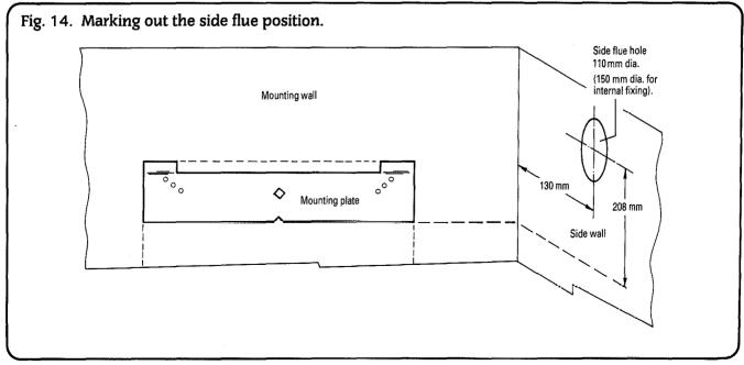
Drill the two fixing holes 60 mm deep for No. 12 size plugs. Cut the flue duct hole at 110 mm diameter (150 mm dia. for internal fitting). Ensure that the hole is horizontal through the wall.
