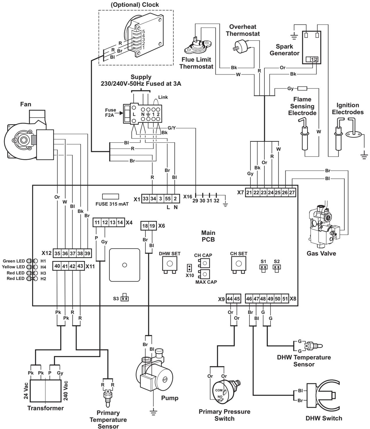
**NOTE:** TO CONNECT EXTERNAL CONTROL REMOVE LINK FROM TERMINALS 1 & 2 AND CONNECT 230/240 V SWITCHED LIVE TO TERMINAL 1.
