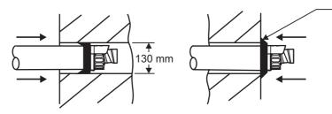
Check collar is sealing the wall and it is not restricting any openings of the flue terminal
