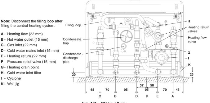
Fig. 14b - With wall jig
