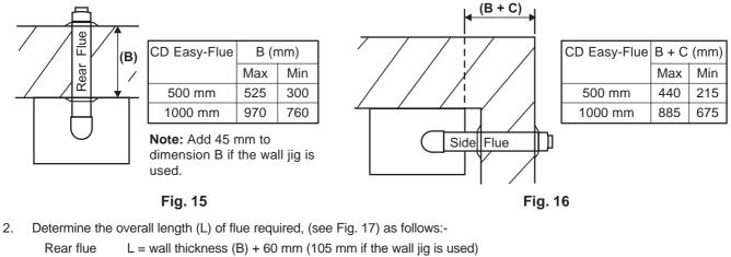
Side flue L = wall thickness (B) + distance between boiler and wall (C) + 145 mm
