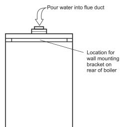
Fig. 13 - rear of boiler
