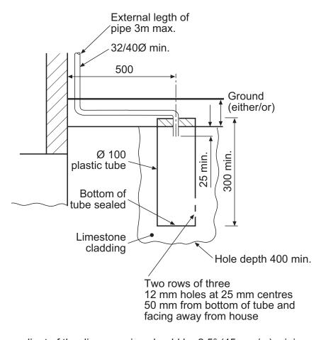
The gradient of the discarge pipe should be 2.5° (45 mm/m) minimum.
