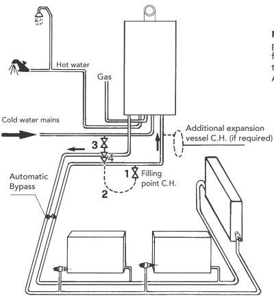
**NOTE:** An automatic bypass capable of passing 6 ltrs per minute must be fitted as far as possible from the boiler if thermostatic radiator valves are fitted thoughout. As per the building regulations part 'L'
