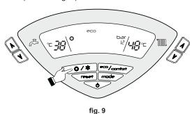
The display activates the Summer symbol (detail 27 - fig. 1): the boiler will only deliver domestic hot water. The frost protection system remains activated.
