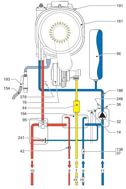
fig. 38 - Water circuit
