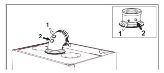
fig. 34 - Flue gas sampling Point
