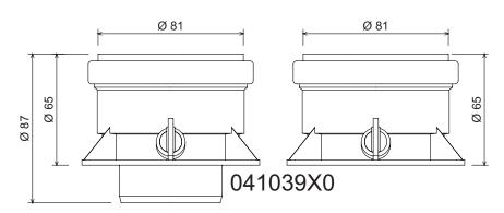
fig. 25 - Starting accessory for separate ducts
