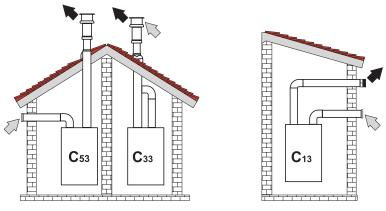
fig. 24 - Examples of connection with separate pipes ( = Air / = = Fumes)
