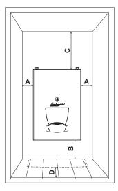
fig. 17 - Minimum distances around the boiler
