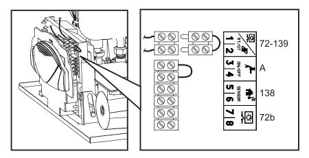
fig. 20 - Electrical terminal block
