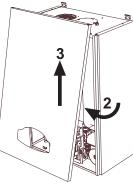
fig. 33 - Opening the casing
