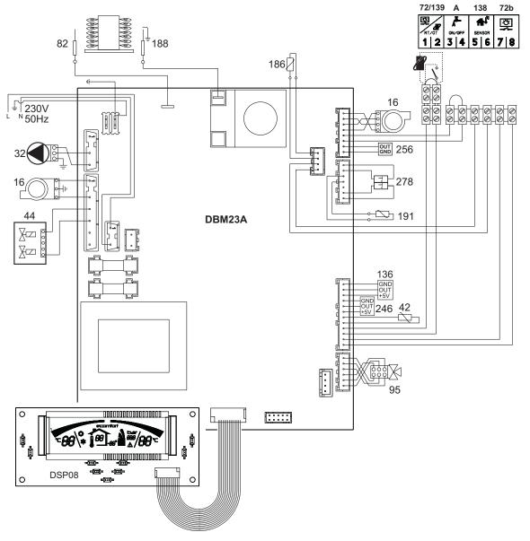
fig. 41 - Wiring diagram
