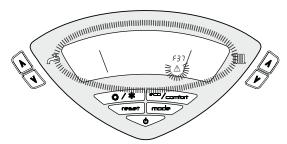
fig. 16 - Low system pressure fault
