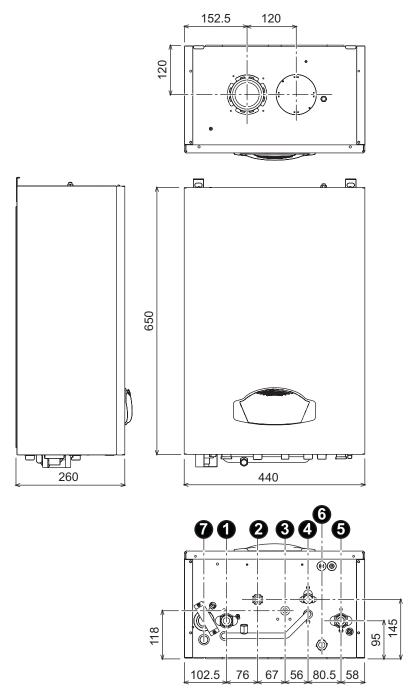
fig. 36 - Dimensions and connections
