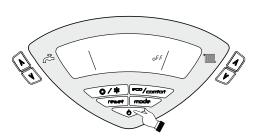
fig. 7 - Turning the boiler off
