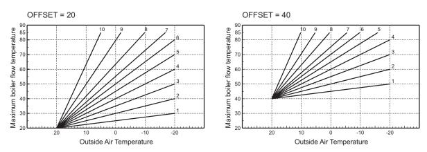
fig. 15 - Example of compensation parallel curve offset
