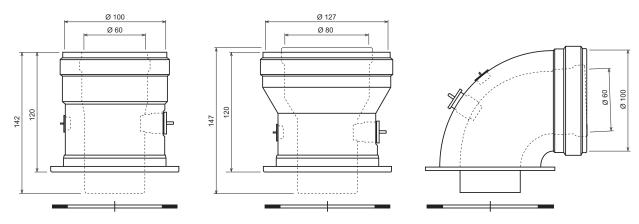
fig. 23 - Starting accessory for coaxial ducts
