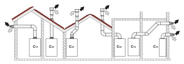
fig. 22 - Examples of connection with coaxial pipes ( = Air / = = Fumes)
