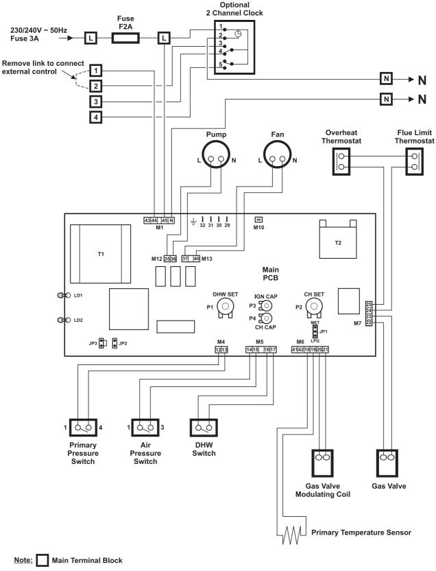
TO CONNECT EXTERNAL CONTROL REMOVE LINK FROM TERMINALS 1 AND 2 AND CONNECT 230/240 V SWITCHED LIVE TO TERMINAL 1.
