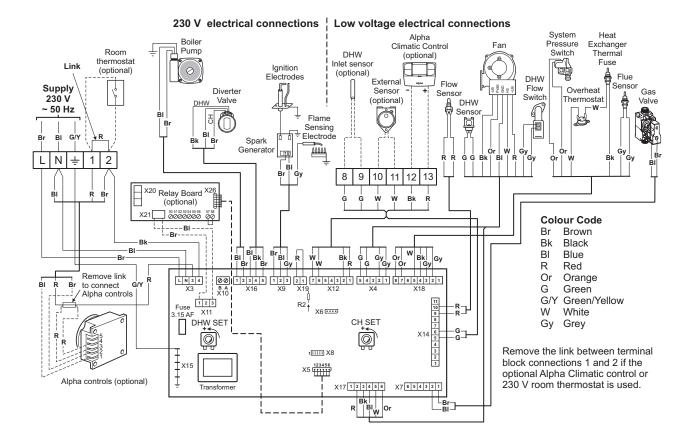
Alpha InTec C and X - Wiring Diagrams 37
