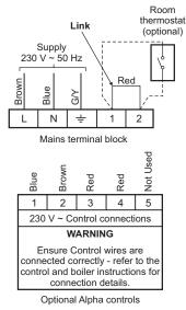
LOW VOLTAGE CONNECTIONS ONLY (optional Climatic or RF Climatic control)
