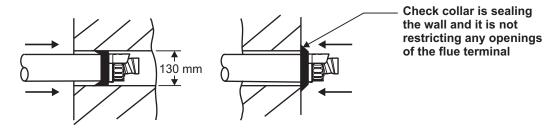
Fig. 17 - Fitting the flue from inside
