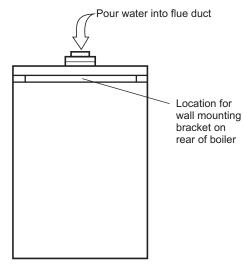
Fig. 12 - rear of boiler
