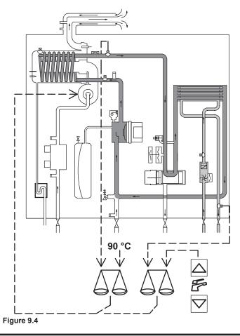
Normally, the result of the comparison between these two signals directly operates the fan speed adjusting the useful output generated in order to stabilize the temperature of the exiting water. If during the d.h.w. mode operation, the temperature of the primary circuit goes over 90°C, the useful output is automatically reduced so that the primary circuit cannot reach excessive temperatures.
