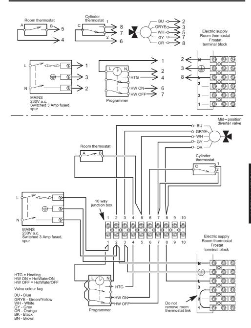
Fig. 6.25 - Not permanent live Y - plan
