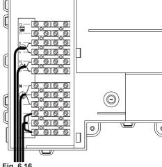
Allow the cables to exit the boiler by using the relevant cable clamps R (Fig. 6.17).
