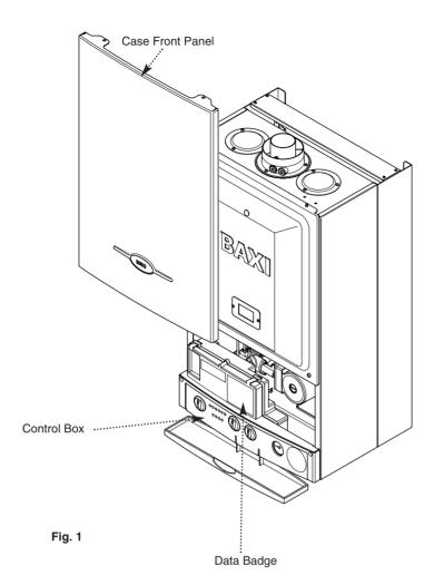
**NOTE:** This appliance must be installed in accordance with the manufacturer's instructions and the regulations in force.
