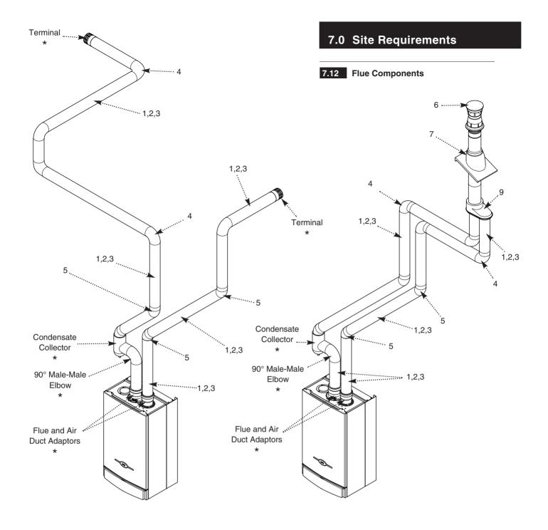
Items marked \* are supplied with each boiler in a separate pack marked
