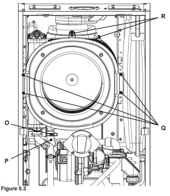
11 Using pliers, remove the spring O moving it downwards and
