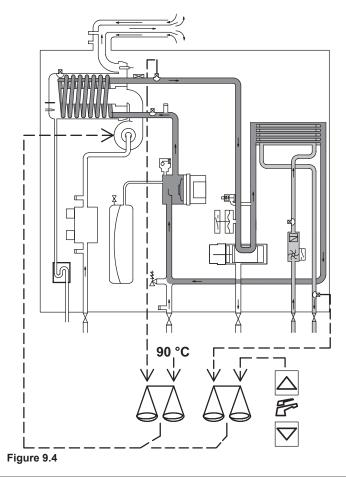
Normally, the result of the comparison between these two signals directly operates the fan speed adjusting the useful output generated in order to stabilize the temperature of the exiting water. If during the d.h.w. mode operation, the temperature of the primary circuit goes over 90°C, the useful output is automatically reduced so that the primary circuit cannot reach excessive temperatures.
