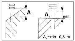
Maximum length of two metre allowed for flue. Ensure terminal position is a minimum distance of 0.3 m from a vertical wall surface or parapet.
