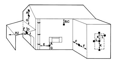
A Quinnell Barratt and Quinnell guard (part. no. C2) should be screwed to the wall centrally over the terminal, when the distance is less than 2 m above a balcony, above ground or above a flat roof to which people have access.
