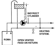
\* h = maximum head developed by pump.
