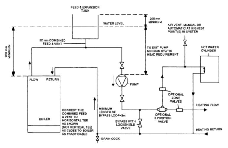
Fig. 4 Fully Pumped Open System - Combined Feed and Vent. (Some water authorities require a stop cock in the cold-feed pipe, in which case this system cannot be used).
