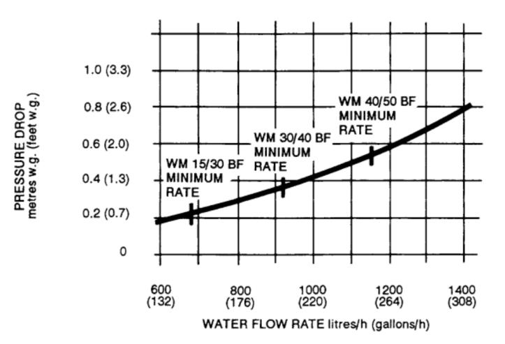
Fig. 3 Resistance to Water Flow through Boiler
