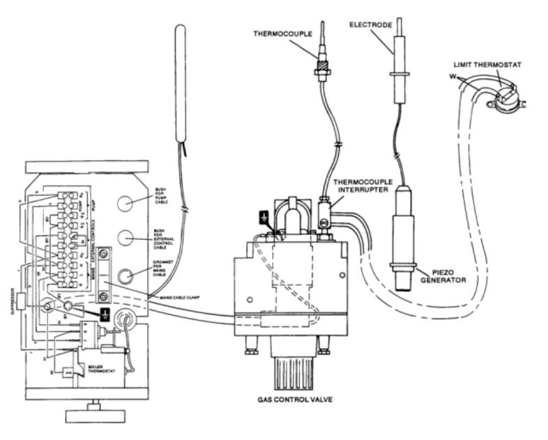
Fig. 8 Control Box Wiring Schematic.
