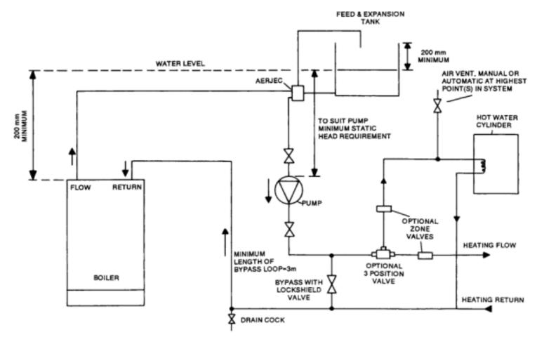
Fig. 5 Fully Pumped Open System - Myson Aerjec. (Improves air removal from system).
