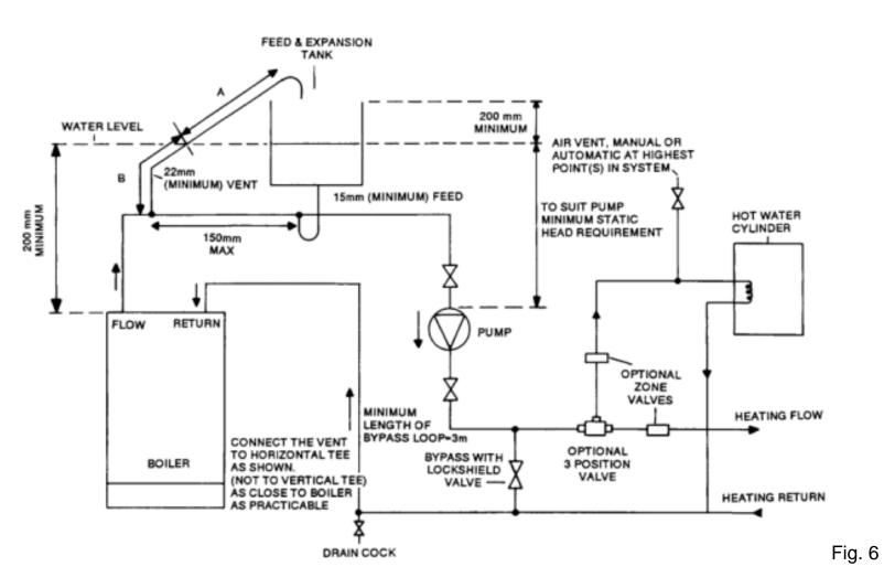
Fully Pumped Open System - Close Coupled Feed and Vent
