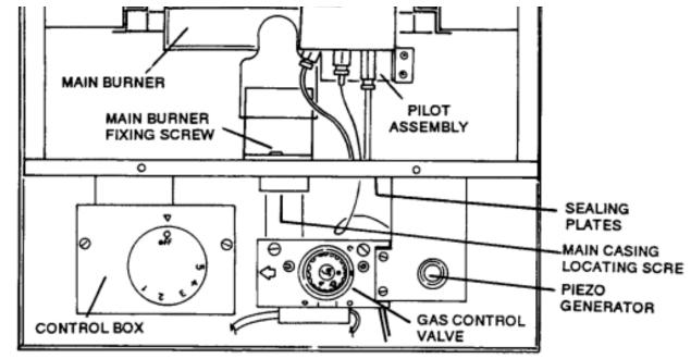
Fig. 13 Internal Layout of Boiler.
