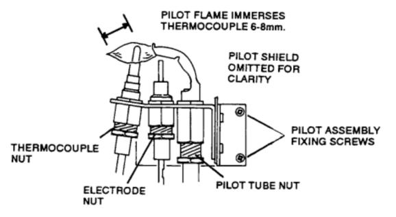
Fig. 14 Details of Pilot Assembly.
