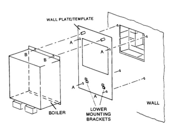
Fig. 10 Boiler Wall Fixing
