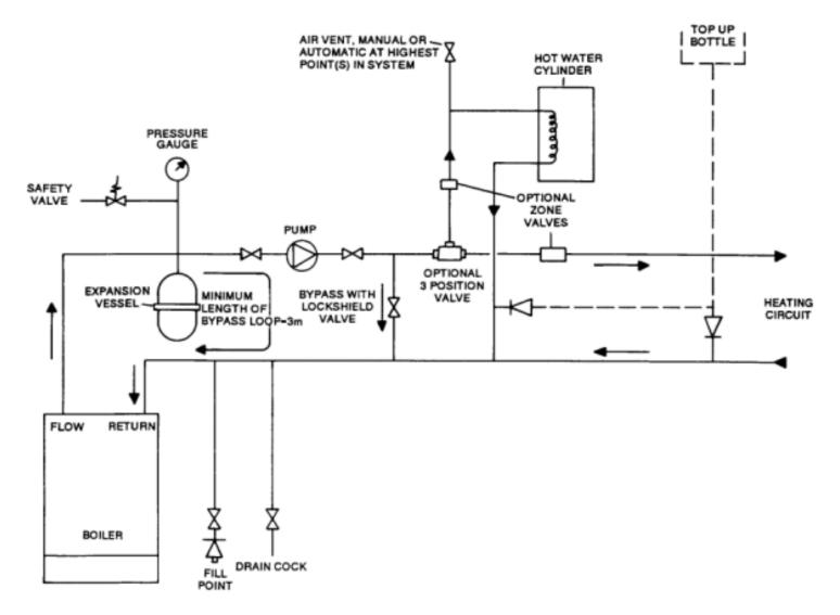
Fig. 7 Fully Pumped Sealed System Piping Diagram.
