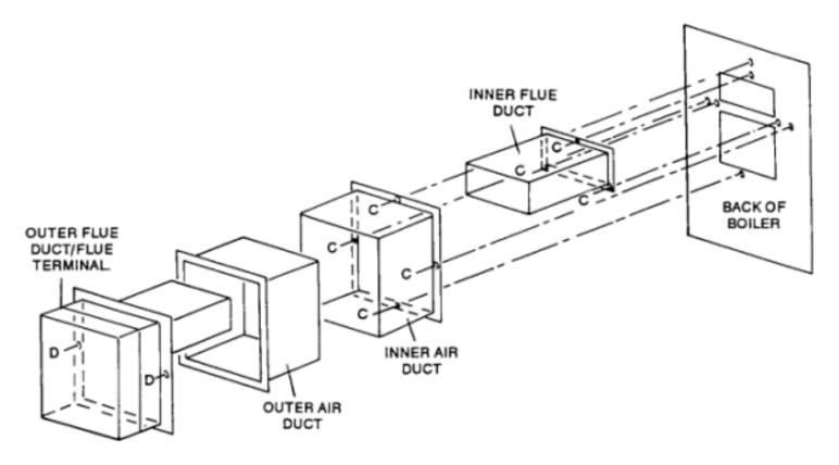
Fig. 11 Flue Duct /Terminal Assembly.
