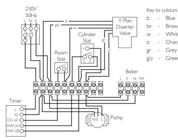
Y Plan, Room Thermostat System, CH Interlocked By Room Thermostat
