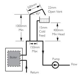
Fig. 10 Typical Low Head Installation
