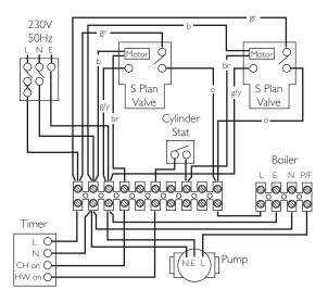
S Plan, Fully TRV'd System, CH Interlocked By Boiler Flow Switch Room Thermostat should not be fitted Pump must be run from Boiler P/F connection for Part L1 compliance
