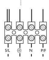
Optional Pump Feed Connection only required for fully TRV'd system
