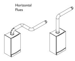
NOTE: Horizontal flue pipes should always be installed with at least a 1.5° fall from the terminal to allow condensate to run back to the boiler.
