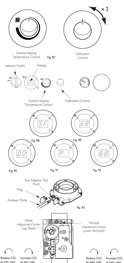
If the CO<sub>2</sub> is reset at minimum rate it must be rechecked at maximum rate again and adjusted if required. If the CO<sub>2</sub> is reset at maximum rate it must be rechecked at minimum rate and adjusted if required.
