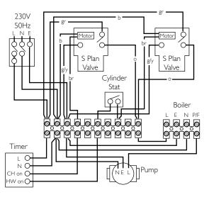
S Plan, Fully TRV'd System, CH Interlocked By Boiler Flow Switch Room Thermostat should not be fitted
