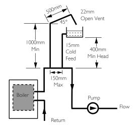
Fig. 10 Typical Low Head Installation
