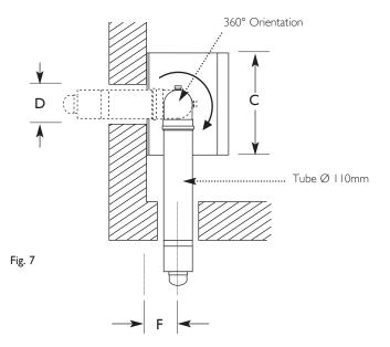
The I.5° fall provided by the elbow is to allow condensate to run back to the boiler, for disposal through the condensate discharge pipe.
