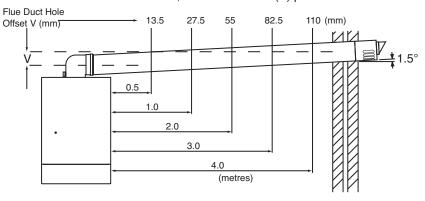
Distance in metres from boiler to the wall. For pipe lengths greater than 4m increase the off-set by 26mm for every additional metre to maintain approx 1.5° inclination.
