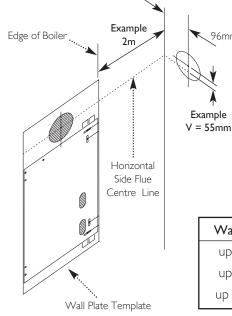
EXAMPLE: Boiler is 2 metres away from corner of wall, flue duct hole is 55mm up from horizontal side flue centre line. This will maintain the approx 1.5° backfall to the boiler.
