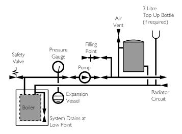
$\label{eq:max-Boiler Flow} \mbox{ Max Boiler Flow} \\ \mbox{Fig. I3} \qquad \mbox{ Temp} = 82^{\circ} \mbox{ C}$
